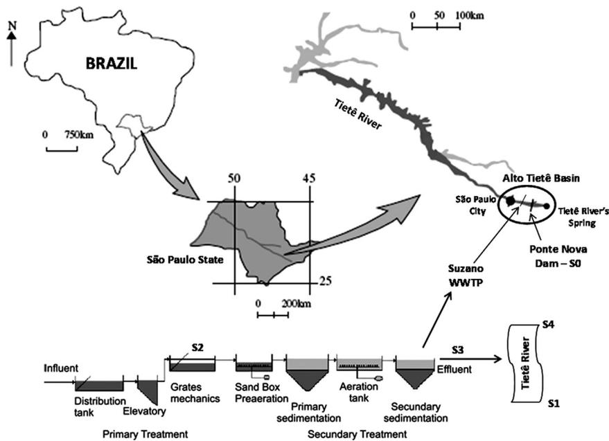
**Fig. 1.** Map showing the Tietê River in São Paulo State (Brazil), Suzano Wastewater Treatment Plant (WWTP), (S0) Ponte Nova Dam (Salesópolis City) and flowchart of the fluid portion of the WWTP with the sites sampled: (S1) 200 m upstream of the plant, (S2) WWTP influent, (S3) effluent and (S4) 200 m from the discharge of the effluent in the Tietê River (Adapted from Cutolo et al. (2006), Rocha et al. (2009)).
